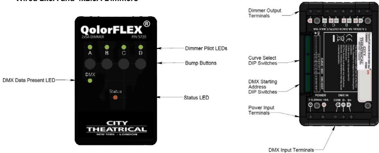
The wired QolorFLEX® 2x5A and 4x2.5A Dimmers have all the same features, except that the 4x2.5A has four dimmer channels (A, B, C & D) while the 2x4A has two dimmer channels (A & B).
