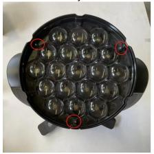
2. Install the standoff with the lock washer.
