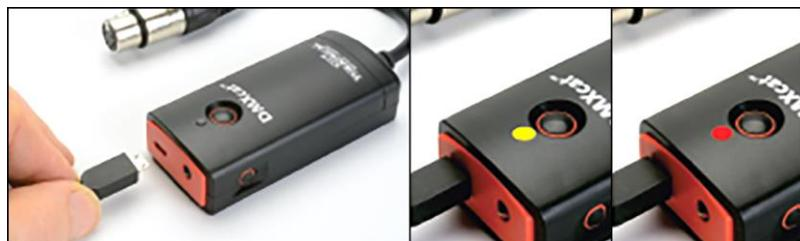
Connect the DMXcat device to a standard 5V DC phone charger using the USB to Micro USB charging cable.
