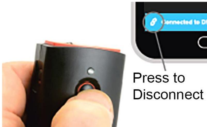
Press the “LINK” icon to disconnect the DMXcat. Press and hold the power button until the LED indicator flashes four times.
