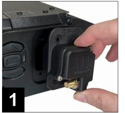
1. Plug the Multiverse Connect Module into the fixture base.
