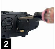
2. Screw the Multiverse Connect Module onto the fixture using a Phillips Head screwdriver and the screws that come with the fixture.
