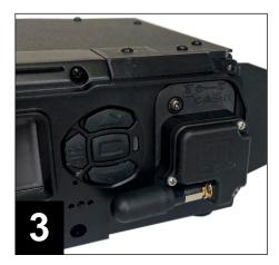
3. Attach the 900MHz antenna to the Multiverse Connect Module, and you're ready to use wireless DMX/RDM with the fixture!
