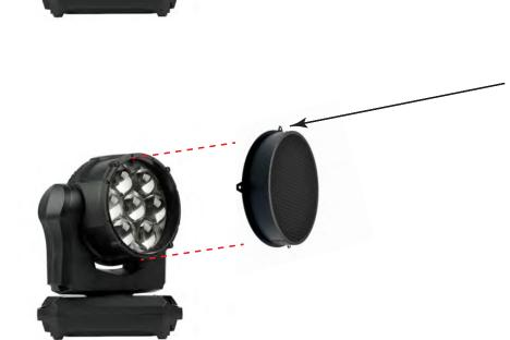
Align accessory with existing screw holes and use (4) original screws to fix accessory to fixture
