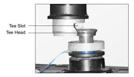
3. Insert the **Tee Head** into the **Tee Slot** manually, such that the Tee Head will settle into the Tee Slot.
