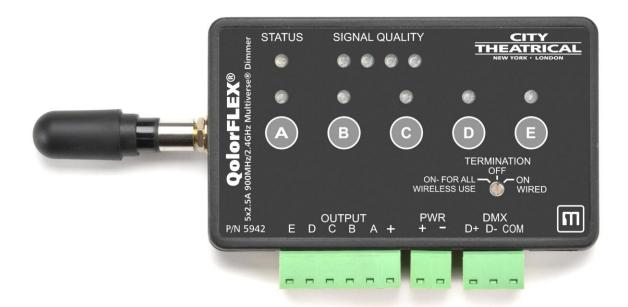
QolorFLEX 5x2.5A 900MHz/2.4GHz Multiverse Dimmer (P/N 5942) is a constant voltage, five-output dimmer that can be controlled wirelessly using City Theatrical's Multiverse or SHoW DMX Neo wireless DMX/RDM technology, or with wired DMX.
