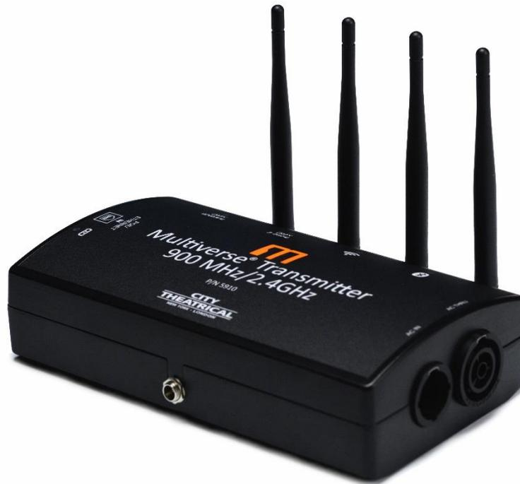
The **Multiverse Transmitter 900MHz/2.4GHz** (P/N 5910) model can broadcast as many as nine universes of DMX data (licensed for use in North America) from a single transmitter, while producing less radio energy than present-day single universe systems.
