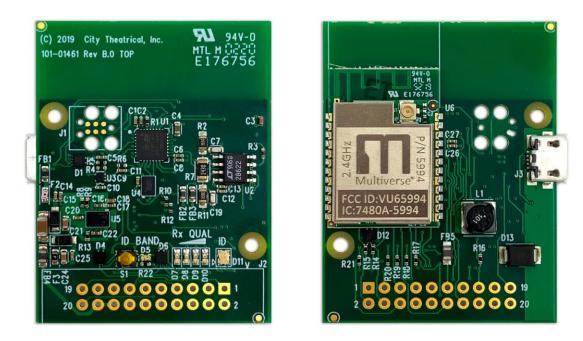
Available in either the 2.4GHz or 900MHz band, City Theatrical's **Multiverse Receiver Card** is a new product that any lighting user can use to implement wireless DMX/RDM into entertainment projects or lighting equipment in a simple way.
