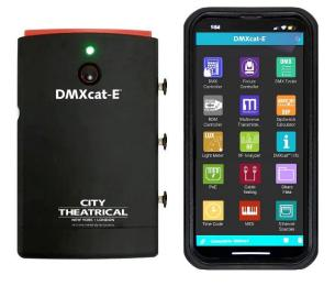
City Theatrical's new DMXcat-E (P/N 6100) allows users to view and send Ethernet protocols, including ArtNet and Streaming ACN (sACN) among others, as well as perform cable testing of 5-pin XLR and Ethernet cables via included external remote.
