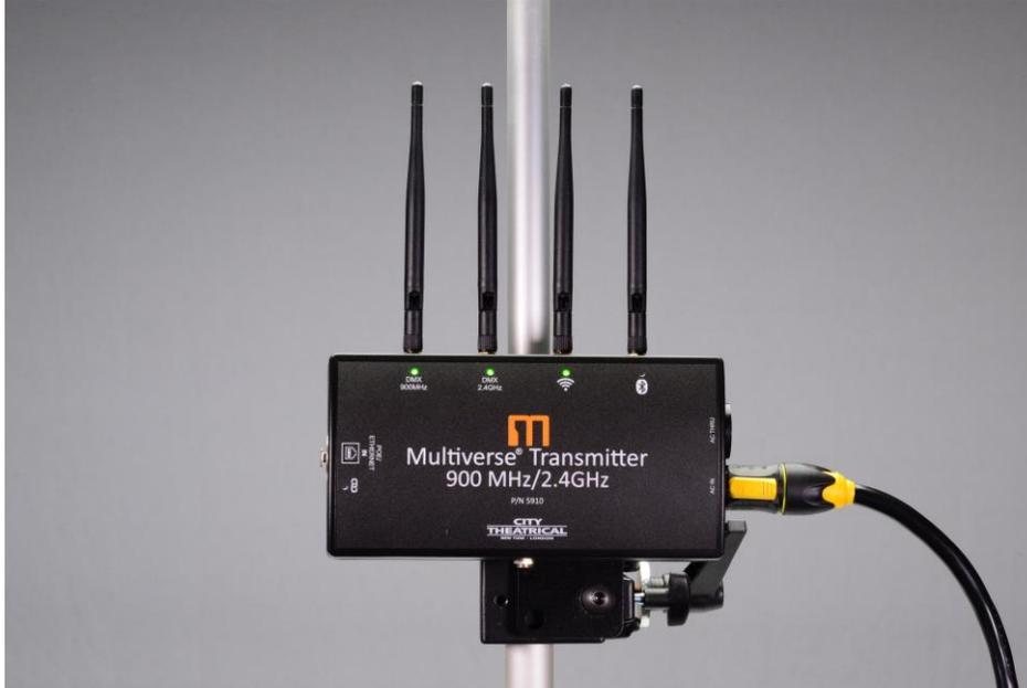
**Multiverse®** wireless DMX/RDM products by City Theatrical, including the **Multiverse Transmitter** (shown), provide a new range of options for performing lighting tasks more easily than ever before, while producing less disruptive radio energy.
