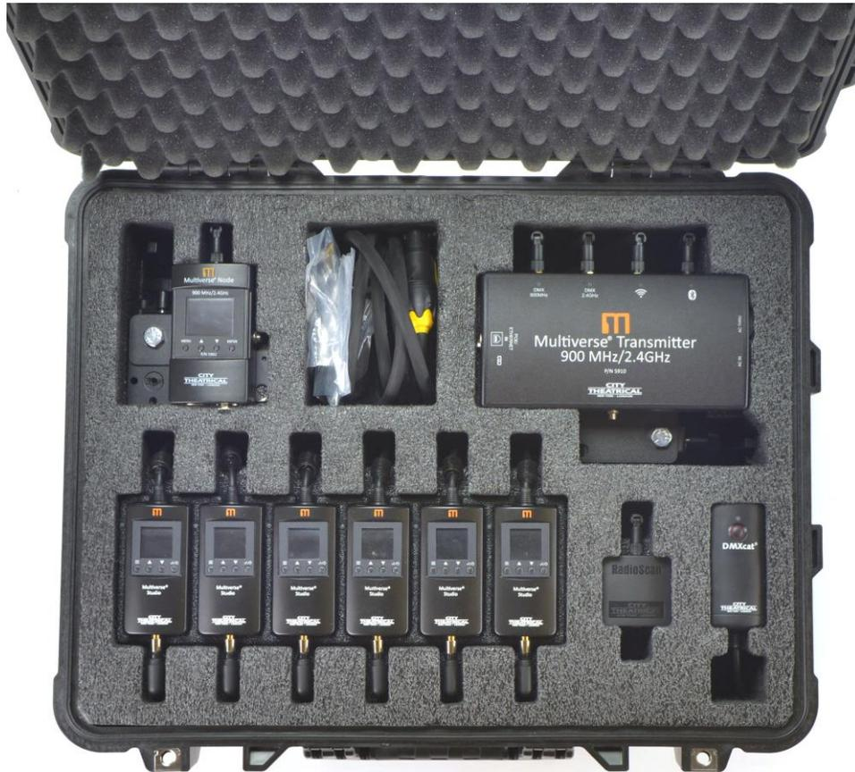
City Theatrical's new Multiverse Studio Kit provides all the tools lighting technicians need to quickly plan, setup, and operate wireless DMX/RDM on set, including: six battery powered Multiverse Studio Receivers, one Multiverse Transmitter, one Multiverse Node, one DMXcat Multi-Function Test Tool, one RadioScan Spectrum Analyzer, and accessories.
