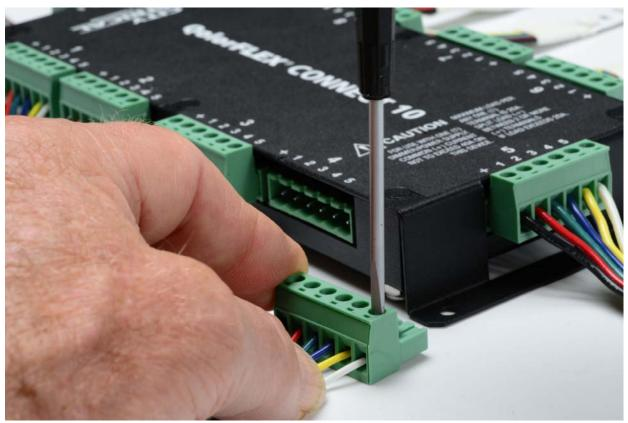
QolorFLEX Connect 10 technology makes setting up large scale LED tape installations faster, and is useful for sets that require assembly multiple times, such as touring productions.
