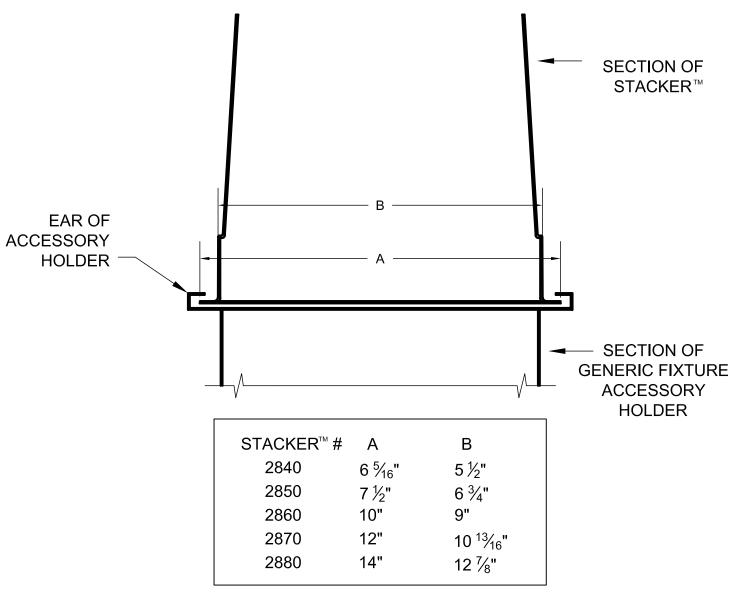
NOTE: CTI's 2850 SERIES STACKERS ™ CURRENTLY DO NOT FIT THE ETC 14°, 70°, OR 90° DUE TO THE ROUNDED CUT ON THE ACCESSORY HOLDER.
