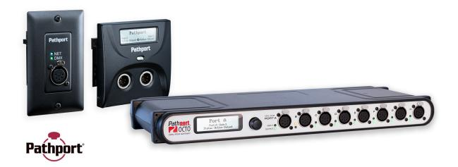
All of Pathway Connectivity's DMX/Ethernet Gateways can receive data from multiple sources at the same time. Data is routed on a slot by slot basis using the free Pathport Manager software. When a port receives data from multiple consoles, it determines which value wins based on the configured Priority.
