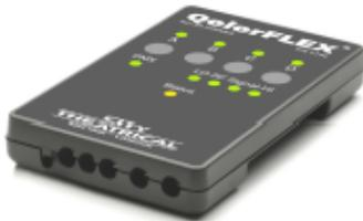
About the size of a credit card and 1/2" (12.7mm) thick, the QolorFLEX™ 2x5A and 4x2.5A Dimmer is a tiny and affordable two channel unit. Designed for controlling LEDs or low voltage incandescent fixtures, it is ideal for use in props, displays, or cabinets where it's size is limited and only two channels of control are required. The QolorFLEX™ 2x5A Dimmer accepts wired DMX data communication from controllers/consols.
