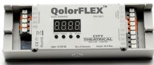
The QolorFLEX™ 4x5A Dimmer can control a full 20A of led tape spread over four channels of 5A each. It uses constant voltage technology which ensures consistent full range of dimming that is especially important at low end light levels. The unit is easily surface mounted and has spring contact terminal blocks for all electrical and data connections.
