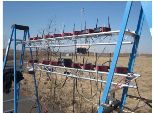
Another view of the 16 Transmitter SHoW DMX rig with the CTI Wireless DMX Tester (blue) in the center of the lower row.
