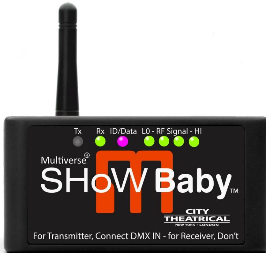
In its default mode, **Multiverse**® **SHoW Baby**™ works like all other SHoW Baby Transceivers with six user selectable SHoW IDs. By connecting an RDM controller, all of the revolutionary new 2.4GHz Multiverse SHoW IDs are accessible as well as all 70 SHoW DMX Neo SHoW IDs.
