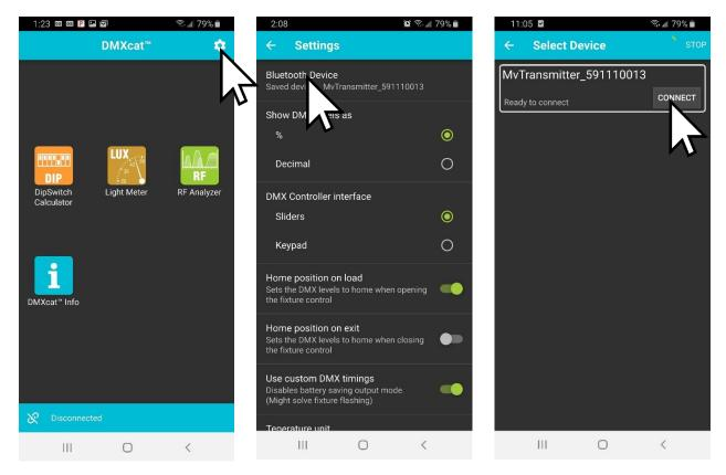
Figure 2: Connecting to Your Multiverse Transmitter with DMXcat
