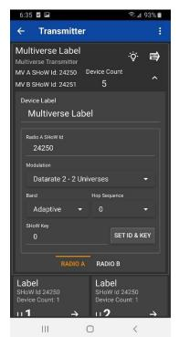
By tapping the drop-down menu arrow, a fuller set of Transmitter options are shown.
