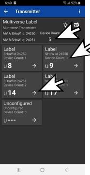
This shows the total number of devices (receivers and lighting fixtures) attached to the Transmitter's two radios.
