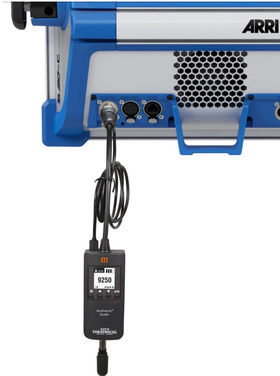
Figure 3: Connected to and Being Powered by USC Cable to Lighting Fixture
