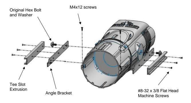
**Note:** If you experience difficultly installing M4x12 screws, it may be due to incompletely threaded holes on the Source Four barrel. Threads can be formed completely with the following steps:
