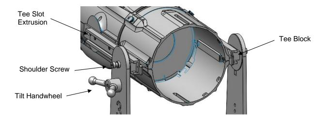
Install four 4-40 x 3/16" pan head machine screws, one in each end of each Tee Slot Extrusion. These screws serve as safety devices to prevent the Tee Blocks from accidentally slipping out of the Tee Slot Extrusion track.
