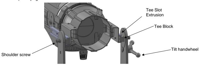
Install four 4-40 x 3/16" pan head machine screws, one in each end of each Tee Slot Extrusion. These screws serve as safety devices to prevent the Tee Blocks from accidentally slipping out of the Tee Slot Extrusion track.
