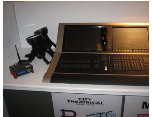
ETC's RDM enabled EOS console, with City Theatrical's SHoW DMX Transmitter at the left.
