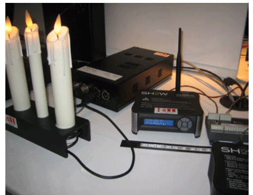
More RDM gear: CTI SHoW DMX Receiver, Howard Eaton RDM Candles, CTI SHoW DMX Dimmer.
