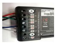
Now, even without DMX, I can use my bump buttons to check my wiring. Plug in the battery. The DMX light will be flashing, showing that DMX is not present. I can press each of the bump buttons to check the circuit and the output of the tape. This allows you to troubleshoot your installation and to track down any wiring errors you may have made (LED tape can be a little confusing sometimes!) before you introduce DMX to the system.
