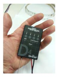
We'll start with one of our D4 Neo Dimmers. This is a four channel dimmer, with a total of 10A of output, and a maximum of 5A on any one channel. You can use four channels of 2.5A each, or three channels of 3.3A each, or two channels of 5A each. I'll be using all four channels.
