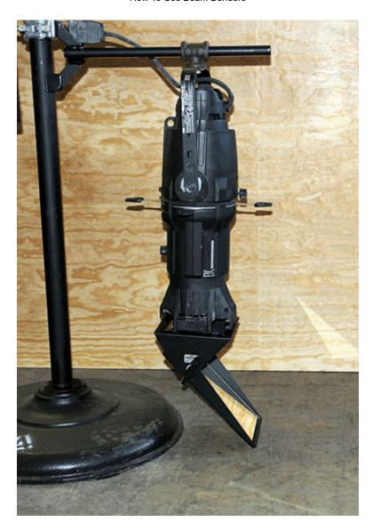
Not all Beam Benders are built with diverting mirrors. We recently created one for designer Rob Schoenbohm of Lightime Design that utilized a prism as a diverter. Here's what Rob told us about how he has used Beam Benders in the past, and how he used them on this particular project:
