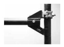
Let's face it, standard theatrical sidearms are poorly designed. They're weak, can't support any downward pressure, and the C-clamp that they use is easily bent and damaged. Our Safer Sidearms eliminate all these problems by adding a strong diagonal brace that transfers force to the vertical boom pipe. These are beautifully engineered devices that will give you years of service.
