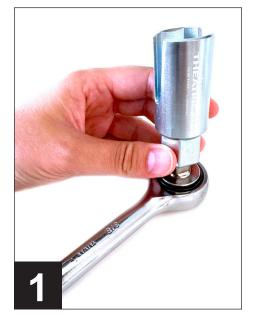
Attach the Wing Nut Socket (City Theatrical Part Number 1305) to a **3/8" ratchet with a push button**, to secure the socket placement.
