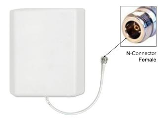
The **7dBi/8dBi Panel Antenna**, **900MHz/2.4GHz**, **Dual Band** (P/N 5981) is a broadband, low VSWR, directional antenna with a 60° Beam spread. While it is designed for for outdoor reception, it can be used for indoor or outdoor projects.
