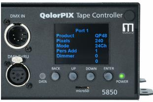
The QolorPIX Tape Controller has a user-friendly control interface that allows the user to change mode, pixel length, dimmer, personality start address, and direction.
