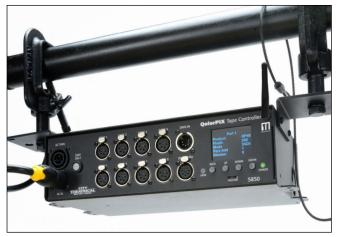
The QolorPIX Tape Controller offers eight ports, each accommodating five metres of tape. It features an integrated power supply, a test function, and flicker finder for easy troubleshooting. It also offers wireless DMX control using City Theatrical's state of the art Multiverse® wireless DMX technology.
