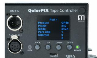
The QolorPIX Tape Controller has a user-friendly control interface that allows the user to change mode, pixel length, dimmer, personality start address, and direction.
