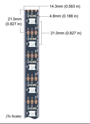
QolorPIX<sup>®</sup> Pixel Controlled LED Tape, IP67-Rated for Outdoor Use Q5050-5-RGB-48-5-67-2
