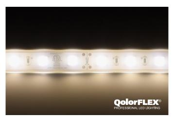
**QolorFLEX LED Tape, Warm White, 24V Outdoor** (P/N 5050-24-WW-60-5-67-1) is an exterior grade 24V LED Tape encased in a clear waterproof silicone sleeve. It has an IP rating of 67 has a high output (900 lumens/ meter) brightness. It is available in full 5 meter reels and sample strips. Waterproof end caps must be used after cutting.
