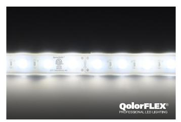
**QolorFLEX LED Tape, Cool White, 24V Outdoor** (P/N 5050-24-CW-60-5-67-1) is an exterior grade 24V LED Tape encased in a translucent waterproof silicone sleeve. It has an IP rating of 67 and a high output (1030 lumens/meter) brightness. The cool white color (6500°K) accentuates blues and subdues greens and reds. It is available in full 5 meter spools and sample strips. Waterproof end caps must be used after cutting.
