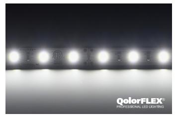
**QolorFLEX LED Tape, Cool White, 24V Indoor (P/N 5050-24-CW-60-5-20-1)** is an interior grade 24V LED Tape with a high output (1030 lumens/meter) brightness. The cool white color (6500°K) accentuates blue and subdues green and red. It is available in full 5 meter spools and sample strips.
