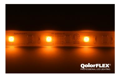
QolorFLEX LED Tape, RGBA, 12V Outdoor (P/N 5050-12-RGBA-60-5-67-1) is an exterior grade hybrid LED tape with a medium output brightness and the ability to create a full spectrum of colors when used with a DMX control system. It is encased in a translucent silicone sleeve which requires the use of end caps after cutting. It is available in full 5 meter spools and sample strips.
