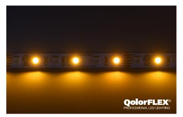
QolorFLEX LED Tape, RGBA, 12V Indoor (P/N 5050-12-RGBA-60-5-20-1) is an interior grade hybrid LED Tape with a medium output brightness and the ability to create a full spectrum of colors when used with a DMX control system. The combination of RGB and amber LEDs allow for precise color mixing for on camera, in studio and theatrical applications. Each LED tape comes with wiring leads on both ends and durable 3M adhesive backing. It is available in full five meter reels and sample strips.
