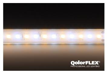
**QolorFLEX LED Tape, Adjustable White, 24V** Outdoor (P/N 3528-24-WWCW-60-5-67-1) is an exterior grade adjustable white LED Tape encased in a translucent waterproof silicone sleeve. It has an IP rating of 67 and the ability to vary the color temperature from very warm (2400°K) to daylight (6500°K) when used with a DMX control system. Its 24V configuration allows for longer runs. It is available in full 5 meter reels and sample strips. Waterproof end caps must be used after cutting.
