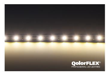
QolorFLEX LED Tape, Warm White, 12V Indoor (P/N **3528-12-WW-60-5-20-1)** is an interior grade LED tape with a medium low output (300 lumens/meter) brightness and a warm 2700°K color temperature. Each LED tape comes with wiring leads on both ends and durable 3M adhesive backing. It is available in full five meter reels and sample strips.
