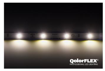
**QolorFLEX LED Tape, Warm White, 12V Indoor (P/N 3528-12-WW-30-5-20-1)** is an interior grade LED tape with a medium low output (150 lumens/meter) brightness in a warm 2700°K color temperature. Each LED tape comes with wiring leads on both ends and durable 3M adhesive backing. It is available in full five meter reels and sample strips.
