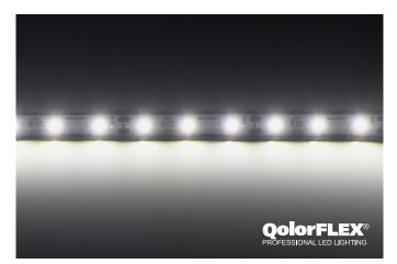
**QolorFLEX LED Tape, Natural White, 12V Indoor** (P/N 3528-12-NW-60-5-20-1) is an economically priced interior grade LED tape with a medium/low output (330 lumens/meter) brightness. Intended for applications where high light output is not required, the natural white color (4100°K) is ideal for use where good color rendition is needed. Each LED tape comes with wiring leads on both ends and durable 3M adhesive backing. It is available in full five meter reels and sample strips.
