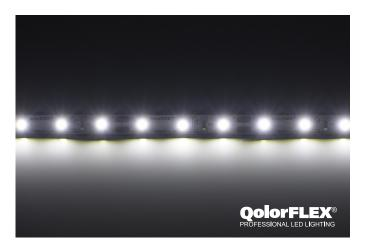
QolorFLEX LED Tape, Cool White, 12V Indoor (P/N 3528-12-CW-60-5-20-1) is an interior grade LED tape with a high output (340 lumens/meter) brightness. The cool white color (6500°K) accentuates blue and subdues green and red. Each LED tape comes with wiring leads on both ends and durable 3M adhesive backing. It is available in full five meter reels and sample strips.
