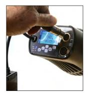
City Theatrical's DMXcat system is designed for use by the lighting professional who is involved with the planning, installation, operation, or maintenance of theatrical and studio lighting equipment. The system consists of a small interface device and a suite of mobile applications. Together, they combine to bring DMX/RDM control plus several other functions to the user's smartphone. DMXcat works with Android, iPhone, and Amazon Fire.
