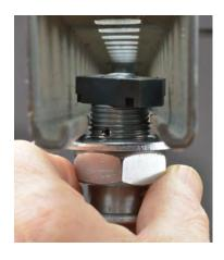
Load-rated City Theatrical Track Tamers separate the lockdown of the track from the lockdown of the lighting fixture, making your job faster and safer.
