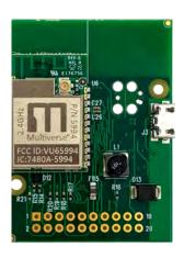
Multiverse Receiver Cards are products that any lighting user, including manufacturers with low volume products, can use to implement wireless DMX/RDM into entertainment projects or equipment, including props, costumes, or lighting fixtures, in a simple way.
