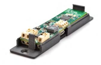
QolorFLEX® 2x2.5A Multiverse® Dimmers are small, constant voltage, two-output dimmers designed to be mounted in small spaces such as props, costumes, wands, and candles.
