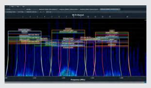
A sample real-life crowded radio spectrum, shown in RadioScan software program.
