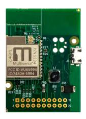
Multiverse Receiver Cards are products that any lighting user, including manufacturers with low volume products, can use to implement wireless DMX/RDM into entertainment projects or equipment, including props, costumes, or lighting fixtures, in a simple way.
