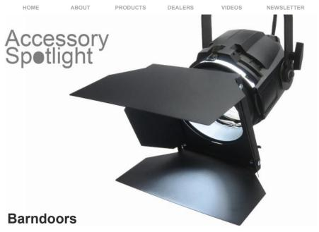
Barndoors are variable beam shaping devices for LED wash lights, fresnels, and Source Four PARs, as seen on the S4 PAR fixture shown. The soft beam of these fixtures has a wide spread without a defined edge, and this wide beam spread often lands on scenery, backdrops, or areas of the stage where it is not wanted. The large leaves of **Barndoors** can be adjusted to shutter the light from these places.
