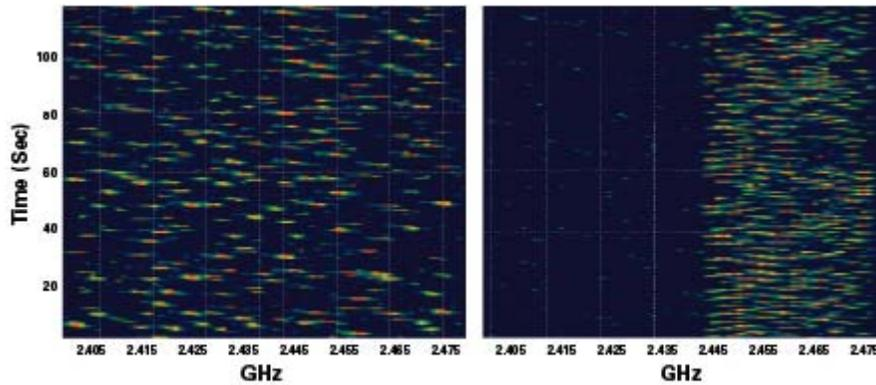
In these Wi-Spy screen shots, the effect of limiting the SHoW DMX bandwidth to WiFi bands 7-12 is clearly shown. In the right hand screen, the portion of the spectrum below 2.466GHz is nearly devoid of activity. Other Wi-Fi signals could operate freely in that area.
