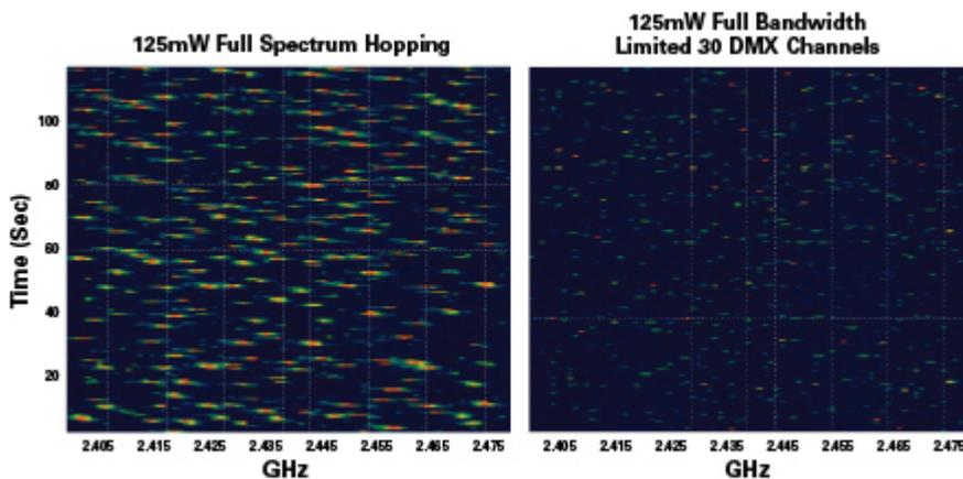
In these screen shots it can be seen that while operating at full power, but limited to an output of 30 DMX channels, SHoW DMX has a very small radio footprint. Some shows don't require all 512 channels to be broadcast via wireless, and this is an excellent option to reduce radio interference with other users in the same venue
