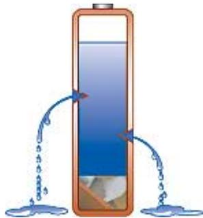
*Figure 3: Effects of high load impedance. Self-discharge increases with age, high cycle count and elevated temperature. Discard a battery if the self-discharge reaches 30% in 24 hours.*
