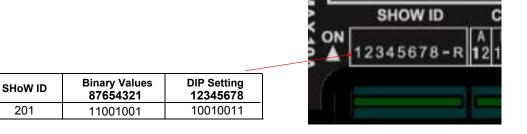
8. Set the DMX Starting Address DIP Switch to the desired starting address, referring to the DMX DIP Switch Tables in the manual.
