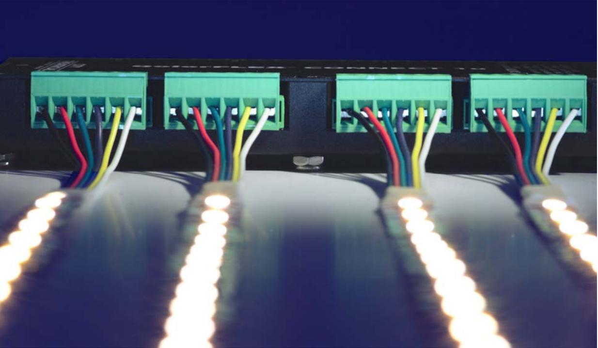
QolorFLEX Connect 10 uses 10 six position detachable Phoenix terminal block connectors to achieve a quick and well-ordered installation.
