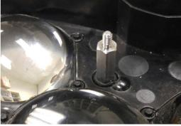
2. Replace M3 Nylon Lock washer with 14mm standoff. Bottom of standoff should come stop after contacting rubber grommet, do not over tighten standoff.
