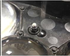
1. Remove the four M3 nylon lock nuts from front of lens, save these parts.
