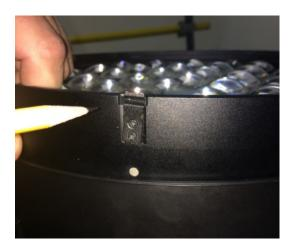
2. Using original screws, attach CTI custom-made tab to the fixture (as pictured below).
